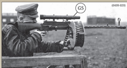
Parabellum LMG 14/17 machine gun of the type carried on LVG C.VI 7243/18 when it was captured on 9 October 1918. Note the Oogje optical sight (G5).
