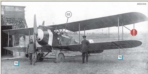
LVG C.VI work number 4507 "K" from Flieger Abteilung (Artillerie) 233 is from the the same production order as 7243/18 C . The cooling slots cut into the nose cowling A1b are not applicable to 7243/18 C .
