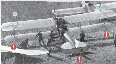
21 An unidentified LVG C.VI reportedly photographed after the Armistice. Note the pale clear doped linen rib tapes.
